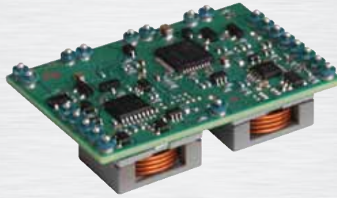
Power Electronics DC/DC Modules
